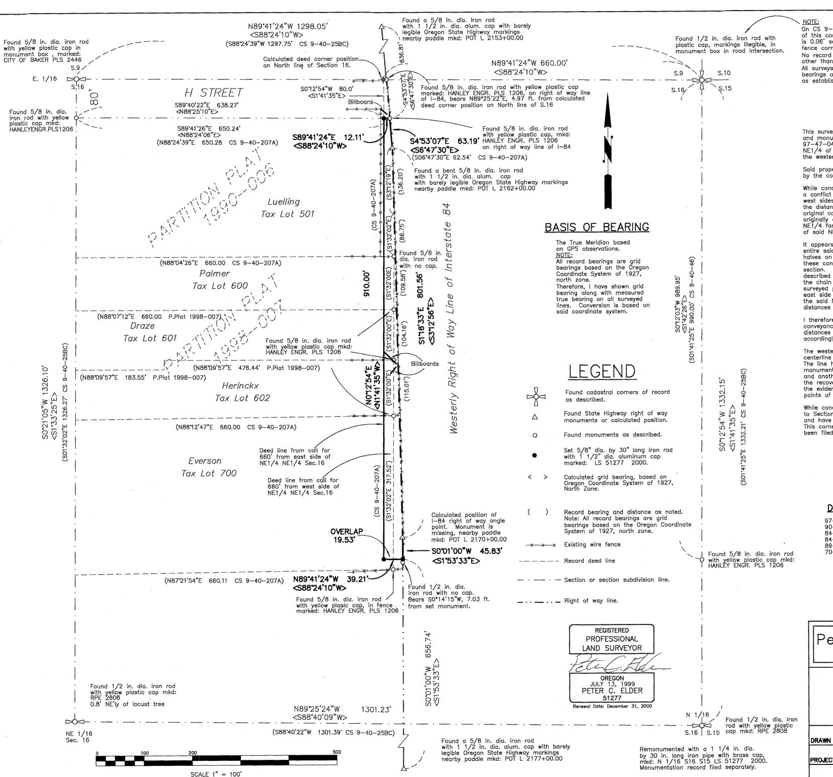
On CS 9-40-394 it is noted that the position of this corner, as remonumented by the city, is 0.06' south and 0.37' east of the accepted fence corner position established in CS 9-40-25BC. No record of the city remonumentation was found other than recognition on subsequent surveys of record. All surveys of record by Hanley Engineering use the bearings of the North and East lines of Section 16 as established by CS 9-40-25BC.
