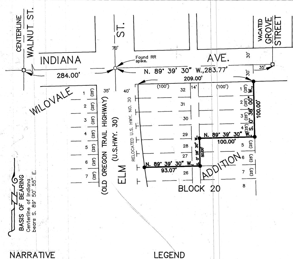
The purpose of this survey for Vernon and Alice Knapp is to mark on the ground with proper monumentation the South and East boundary of their property. The West boundary line is the East right of way line of relocated U.S. Highway No. 230. The North boundary line is the South line of Indiana Avenue. Reference is made to Deeds 84 40 081, 86 48 012 and 96 52 053.
