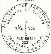
Painted a 6 inch red band around the bearing tree, and also painted the blaze red. Attached USFS 54-3 and 54-9 signs to the bearing tree.
