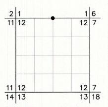
ORIGINAL DESCRIPTION: Set an ironstone 15 x 8 x 6 ins. 10 ins. in the ground, for 1/4 sec. cor., marked 1/4 on N. face, from which A yellow pine, 32 ins. diam., bears N.25°E., 58 lks. dist., marked 1/4 S., B.T.; A yellow pine, 32 ins. diam., bears S.30½°W., 29 lks. dist., marked 1/4 S., B.T.
