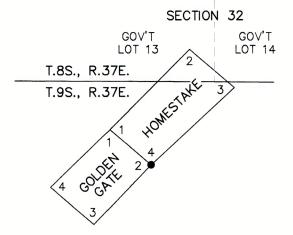
**ORIGINAL DESCRIPTION:** A pine post 4 ft. long, 4 ins square set 18 ins in the ground, surrounded with a mound of earth and stone, scribed Homestake 4-514 and Golden Gate-2-514 Identical with location S.E. cor. post. From which
