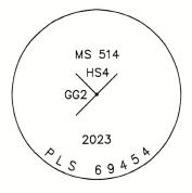
Painted a 6 inch red band around the bearing tree, painted the blazes red, and attached USFS 54-3 and 54-9 signs. Used a total station to measure accessories. Distance to BT was measured to a 60d nail driven in the side-center-right at the base of the tree, with an attached  $1\frac{1}{2}$ " aluminum washer stamped PLS 69454. Set aluminum post N.47°E., with USFS signs 54-2 and 54-9 attached. See associated Map of Survey dated October 17, 2023 for survey-related information.
