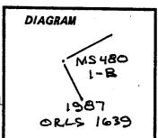
Corner REMONUMENTED by L.L.Myers, ORLS 699, in 1970 as described in his record filed with the Baker County Surveyor (No. 9-36-7), on Aug.31,1977, which states: "I found a rock mound with a small stake marking the corner. The original post was gone as were the bearing trees. Set a 5/8" x 30" rebar with a 2" aluminum cap in the rock mound marked as shown above. This survey did not tie to the range line and section corner as the original did."
