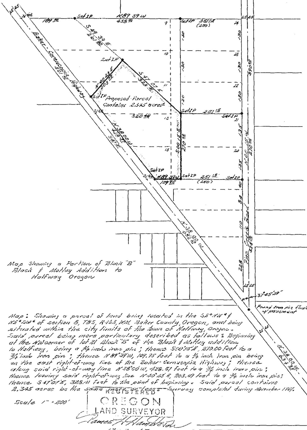
Basis of True meridian is taken from the 1820 bearing along the sec line between sections 9 & 17 T8S R46E W4.
