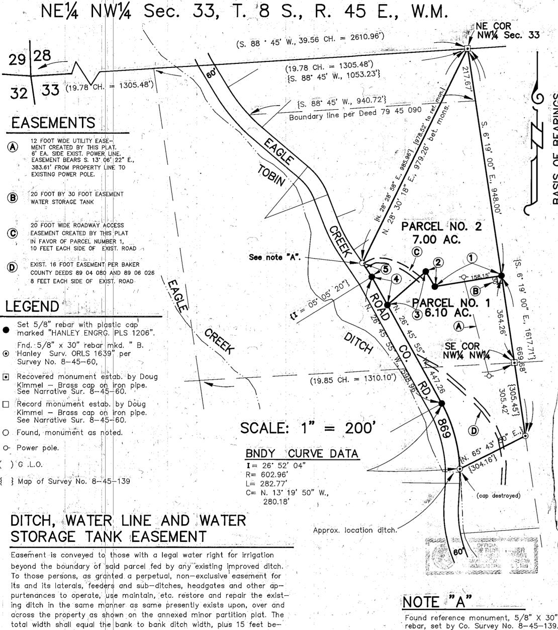
rebar, set by Co. Survey No. 8-45-139. Rebar was disturbed but not replaced. Rebar now located N. 25' 15' 12" E., 6.71 feet from true corner position. The rebar was bent so Wayne Miller straightened it out and drove a large iron plumbing cap on top of it.
