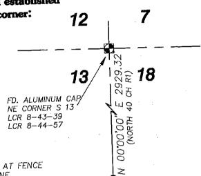
SET  $\frac{5}{8}$ " X 30' STEEL PIN WITH CAP PLS 66818 AT FENCE INTERSECTION IN THE LOCATION OF FOUND STONE.
