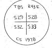
.I used a steel tape and magnetic compass in the establishment of the accessories. I stated a declination of 20° East.
