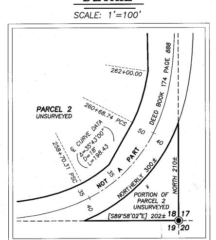
A SEARCH WAS MADE OF THE AVAILABLE RECORDS PERTAINING TO THIS SURVEY. THE POSITIONS OF THE SW AND SE CORNERS OF SECTION 18 WERE ESTABLISHED IN RECORD SURVEY NO. 8-42-3, AND THEN LATER REMONUMENTED BY THE COUNTY SURVEYOR IN 1995. I RECOVERED BOTH OF THESE MONUMENTS DURING
