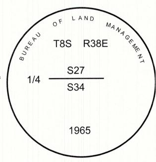
I used a steel tape and magnetic compass in the establishment of the new accessories. I used 14° East declination, the distances are to the center of the chiseled 'X'.
