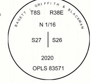
I used a steel tape and magnetic compass in the establishment of the new accessories. I used 14° East declination, the distances are to a 60d spike driven into the right side of the root crown of the bearing trees. A brass washer marked OPLS 83571 is attached to the BT blaze of the new bearing trees.
