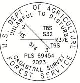
Placed a plastic-encased magnet beneath the base of the aluminum pipe. Used RTK GPS to measure the reference points. Set an aluminum guard post East, 3.0 ft., with USFS 54-2 and 54-9 signs attached, and another S.49°E., 3.3 ft., with USFS 54-2 sign attached. See associated Map of Survey dated October 17, 2023 for survey-related information.
