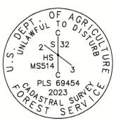
Placed a plastic-encased magnet beneath the base of the aluminum pipe. Used a total station to measure the reference points. Set an aluminum guard post North, 3.8 ft., with USFS 54-2 and 54-9 signs attached, and another N.49°W., 2.5 ft., with USFS 54-2 sign attached. See associated Map of Survey dated October 17, 2023 for survey-related information.
