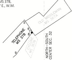
**ORIGINAL DESCRIPTION:** Set a white fir post 4 ins. square  $4\frac{1}{2}$  ft. long 18 inches in the ground with a mound of earth around it marked TEL C7- 378
