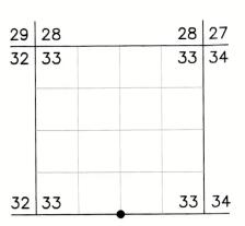
**ORIGINAL DESCRIPTION:** Set an iron post, 3 ft. long, 1 in. dia., 27 ins. in the ground, for 1/4 sec. cor. of sec. 33 only, with brass cap marked (diagram shown) from which
