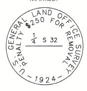
Painted a 6 inch red band around each bearing tree, painted the blazes red, and attached USFS 54-3 and 54-9 signs. Used a staff compass with 14° East declination to measure bearings to BT's. Used an EDM device to measure distances to new bearing trees, measuring to a 60d nail driven in the side-center-right at the root crown of each tree, with an attached  $1\frac{1}{2}$ " aluminum washer stamped PLS 69454. See associated Map of Survey dated October 17, 2023 for survey-related information.
