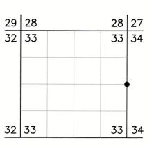
**ORIGINAL DESCRIPTION:** Set an iron post, 3 ft. long, 1 in. dia, 27 ins. in the ground, for 1/4 sec. cor., with brass cap marked (diagram shown) from which
