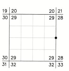
**ORIGINAL DESCRIPTION:** Set an iron post, 3 ft. long, 1 in. dia., 27 ins. in the ground, for 1/4 sec. cor., with brass cap marked (diagram shown) from which
