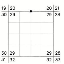
**ORIGINAL DESCRIPTION:** Set an iron post, 3 ft. long, 1 ins dia., 27 ins. in the ground, for  $\frac{1}{4}$  sec. cor., with brass cap marked (diagram shown) from which
