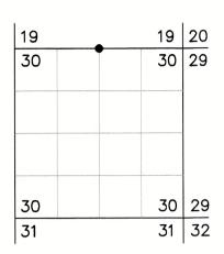
**ORIGINAL DESCRIPTION:** Set an iron post, 3 ft. long, 1 ins dia., 27 ins. in the ground, for  $\frac{1}{4}$  sec. cor., with brass cap marked (diagram shown) from which
