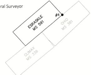
**ORIGINAL DESCRIPTION:** To Cor. No. 4 A tamarack post 4 ft long, 4 ins square, set 18 ins in the ground, surrounded with a mound of earth & stone and marked Esraskle-4-591 Identical with location S.E. cor. post. From which A pine 10 ins in diam. bears S27°40'E 1.6 ft. dist. marked Esraskle-4-591-B.T. A fir 6 ins in diam. bears N15°30'W 6.7 ft. dist. marked -4-591-B.T.
