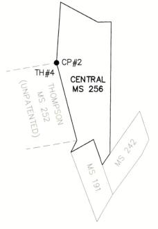
**EVIDENCE FOUND:** Found Mitchell's unrecorded monument, which is a  $1\frac{1}{2}$ " galvanized iron pipe with a  $2\frac{1}{2}$ " brass cap, marked as shown, projecting 1" above ground in a 3 ft. diameter mound of stone. From the found brass cap monument, I also found the following bearing trees:
