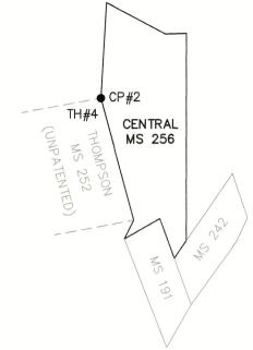
ORIGINAL DESCRIPTION: To corner No. 4. Set a post 4½ feet long 4 inches square, 12 inches in the ground with mound of stone, marked Cor. 4 T.Q.C. from which N.E location corner bears N.13°E. 96 feet distant. A Fir 18 inches dia, blazed and marked Cor. 4 T.Q.C. B.T. bears West 39 feet distant. A Fir 20 inches dia, bears S.65°W. 37 feet distant marked B.T.
