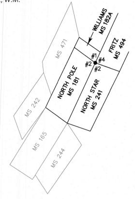
**ORIGINAL DESCRIPTION:** To corner No. 2. Set a black pine post 5 ft  $\lg 4 \frac{1}{2}$ " square 12" in the ground marked cor No. 2 NPMC S No. 181 with a mound of stone around it from which
