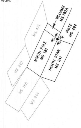
**EVIDENCE FOUND:** Found Mitchell's unrecorded monument, which is a  $1\frac{1}{2}$ " galvanized iron pipe with a  $2\frac{1}{2}$ " brass cap, marked as shown, which was disturbed by logging activity and leaning downhill. I reset the monument and rebuilt a 2 ft. diameter mound of stone to top of cap. From which,
