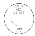
Painted a 6 inch red band around each bearing tree, and also painted blazes red and attached USFS 54-3 and 54-9 signs. Bearings were measured with a handheld compass with a  $14^{\circ}$  East declination. Distance to bearing trees was measured with a steel tape. The new BT was measured to a 60d nail driven in the right-side-center above the root crown with a  $1\frac{1}{2}$ " aluminum washer stamped PLS 91693.
