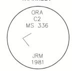
Painted a 6 inch red band around each bearing tree, and also painted blazes red and attached USFS 54-3 and 54-9 signs. Bearings were measured with a handheld compass with a 14° East declination. Distance to bearing trees was measured with a steel tape. The new BT was measured to a 60d nail driven in the right-side-center above the root crown.
