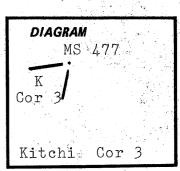
Description of corner evidence found: Found a mound of earth with the remains of a rotted post underground from which: A 9" down lodgepole pine bears S70 3/4°E-12.8' with scribing visible on open
