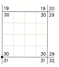
**ORIGINAL DESCRIPTION:** Set an iron post, 3 ft. long, 2 ins dia., 27 ins. in the ground for closing cor. of secs. 30 and 31, with brass cap marked (diagram shown) from which
