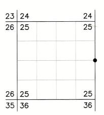
**ORIGINAL DESCRIPTION:** Set an iron post, 3 ft. long, 1 in. dia., 27 ins. in the ground, for 1/4 sec. cor. of sec. 25 only, with brass cap marked (diagram shown) from which
