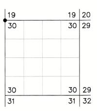
**ORIGINAL DESCRIPTION:** Set an iron post, 3 ft. long, 2 ins dia., 27 ins. in the ground, for closing cor. of secs. 19 and 30, with brass cap marked (diagram shown) from which
