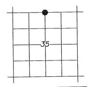
ORIGINAL G.L.O. DESCRIPTION: Set a basalt stone 18x10x8 ins 10 ins in the gro., for the 1/4 sec. cor. marked ¼ S. on the N. face and raised a mound of stone 3 ft. base 24 ins., high 10 lks N. of the cor.
