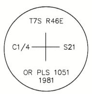
Painted a 6 inch red band around each bearing tree, and also painted blazes red and attached USFS 54-3 and 54-9 signs as needed. Distances to new reference monuments measured with steel tape. Distances to bearing trees measured with handheld EDM. Bearings measured with a handheld compass with 14° East declination.
