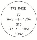
Painted a 6 inch red band around Barbour's bearing trees, and also painted blazes red. Used a magnetic compass with 14° East declination to measure bearings to BT's. Distances measured with a steel tape.
