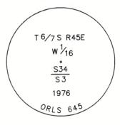
Rebuilt the mound of stone, 3 ft. diameter base to top of cap. Painted a 6 inch red band around the bearing trees, and also painted blazes red. Used a staff compass with 14° East declination to measure bearings to BT's. Distances were measured with a steel tape, measuring to a 60d nail driven in the side-center-right at the root crown of each tree, with an attached  $1\frac{1}{2}$ " aluminum washer stamped *PLS 69454*. Attached new USFS 54-3 signs to BT's with updated information.
