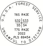
Painted a 6 inch red band around the bearing tree, and also painted blazes red. Attached USFS 54-3 and 54-9 signs to BT. Distance to bearing tree was measured with a steel tape to a 60d nail driven in the side-center at the root crown of the tree, with an attached 1½" aluminum washer stamped PLS 69454. Used RTK GPS to measure accessories. Bearings are geodetic, derived by GPS observation at the corner. Set an aluminum guard post North, 2.5 ft. with USFS 54-2 and 54-9 signs attached.
