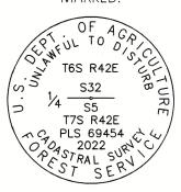
Deposit marked stone inverted, with K-tag and boundary sign Northeast and alongside the pipe. Used RTK GPS to measure accessories. Bearings are geodetic, derived by GPS observation at the corner. Set an aluminum guard post East, 3.8 feet with USFS 54-9 sign attached.
