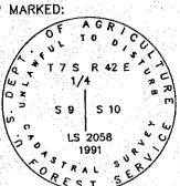
FROM WHICH G.L.O. & H.E.S. ACCESSORIES: A PINE STUMP, 24" DIAM. [16"] (24"), BEARS S60"W [S60'E] (S58'W), 6.6' [6.6'] (6.6'). FROM WHICH LS2058 ACCESSORIES A PINE, 7" DIAM. BEARS S76"30"E, 9.1", SCRIBED "1/4S10BT A PINE, 6" DIAM. BEARS N73'08'W, 7.08', SCRIBED "1/4S9BT" A PINE, 10" DIAM. BEARS N23'36'W, 18.39', SCRIBED "1/4S9BT" A PINE, 8" DIAM. BEARS N16"25'E, 26.30', SCRIBED "1/4S10BT"
