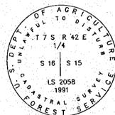
FROM WHICH LS2058 ACCESSORIES: AN + CHISELED IN 25'X40'X5' LEDGE ROCK BEARS S25'10'W, 32.44'. AN + CHISELED IN 10'X5'X2' LEDGE ROCK BEARS N36'56'W, 33.14'. AN + CHISELED IN 1'X1'X1' LEDGE ROCK BEARS
