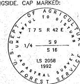
FROM WHICH LS2058 ACCESSORIES: A 1/2" REBAR/ALUMINUM CAP BEARS N5114'W, 24.60' A 1/2" REBAR/ALUMINUM CAP BEARS N48'48'E, 32.31' A PINE, 17" DIAM. BEARS S81'22'E, 72.21', SCRIBED "1/4S16BT" A PINE, 14" DIAM. BEARS S46'36'W, 61.84', SCRIBED "1/4S9BT"
