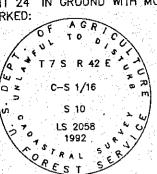
FROM WHICH LS2058 ACCESSORIES: A FIR, 18" DIAM. BEARS S28'27'W, 17.01', SCRIBED "C-S1/16S10BT" A FIR, 10" DIAM. BEARS S33'59'E, 28.22', SCRIBED "C-S1/16S10BT"
