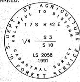
FROM WHICH G.L.O. ACCESSORIES: A PINE, 28" DIAM. [18"], BEARS S27E [S27E], 24.4" [24.4'], WITH PARTLY OPEN BLAZE, SCRIBING VISIBLE. FROM WHICH LS2058 ACCESSORIES A PINE, 10" DIAM. BEARS N54'42'E, 16.73', SCRIBED "1/4S3BT A FIR, 14" DIAM. BEARS N16'55'W, 25.06', SCRIBED "1/453BT" A FIR, 20" DIAM. BEARS \$89"10"W, 15.88", SCRIBED "1/4SBT"
