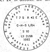
FROM WHICH LS2058 ACCESSORIES: A PINE, 9" DIAM, BEARS N84'05'E, 1.60', SCRIBED "C-N-S 1/64S10BT" A FIR, 13" DIAM. BEARS NO3'04'W, 33.65', SCRIBED "C-N-S 1/16510BT"
