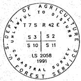
FROM WHICH G.L.O. ACCESSORIES: A PINE STUMP, 24" DIAM. BEARS N64W 26.4' [N64W 26.4'] A TAMARACK, 20" DIAM. [15"], BEARS S32W [S32W], 27.1' [27.1'] BLAZE VISIBLE ON FALLEN AND ROTTED TREE A STUMP HOLE [PINE 30" DIAM.], BEARS SOJE [SOJE]. 46.9' [46.9']
