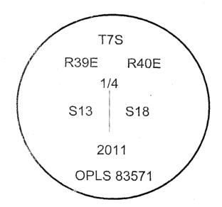
I used a Leica 1200 RTK GPS in the establishment of the accessories. Basis of bearings is a solar observation taken at a point 3550 feet South and 3360 feet West of the Northeast corner of Section 22, Township 6 South, Range 39 East of the Willamette Meridian. Bearings and distances are to the center of the aluminum cap accessories.
