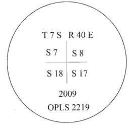
I used a steel tape and magnetic compass in the establishment of the new accessories. I used  $18^{\circ}$  East declination, the distances are to a center of the aluminum cap.
