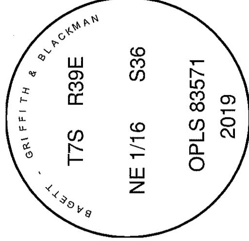
I used a Leica GS-18 RTK GPS in the establishment of the accessories. Bearings and distances are to the center of the aluminum caps. Basis of Bearings is as per Survey for McEst Ranches, as filed with the Baker County Surveyor.
