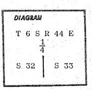
A pine 8 ins. diam. bears N 80° W, 95 lks dist. marked 1/4 S BT A pine 4 ins. diam. bears S 75° E, 55 lks dist. marked 1/4 S BT
