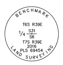
Used RTK GPS to measure the reference points. See associated survey dated July 22, 2016, filed separately.
