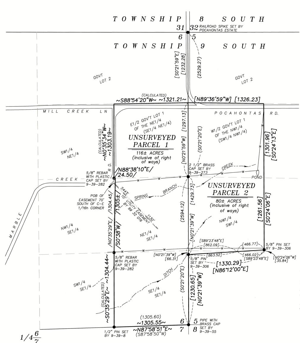
LEGENDSurvey monument of record, as described, not tied by this partition Approximate location of ditch or creek, placed by Lidar data dated 2012 or aerial photograph Approximate location of mainline, shown as per Partition Plat 1998-006 Easement Line Record measurement as per Survey 9-39-08 Record measurement as per Survey 9-39-282 Record measurement as per Survey Bearing and distance calculated from Survey Number 9-39-26 Record measurement as per deed B15 10
